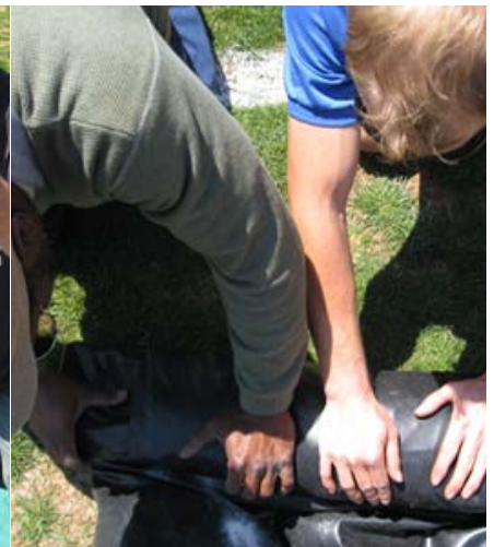
Step 7: Begin rolling from opposite the Blower tube end. (This pushes air out as you roll.) Take your time and roll as tightly as possible. Keep the roll lined up, tuck any in extra material, as you go and do not allow any part of the roll to sag. Loose rolls are difficult to move.
