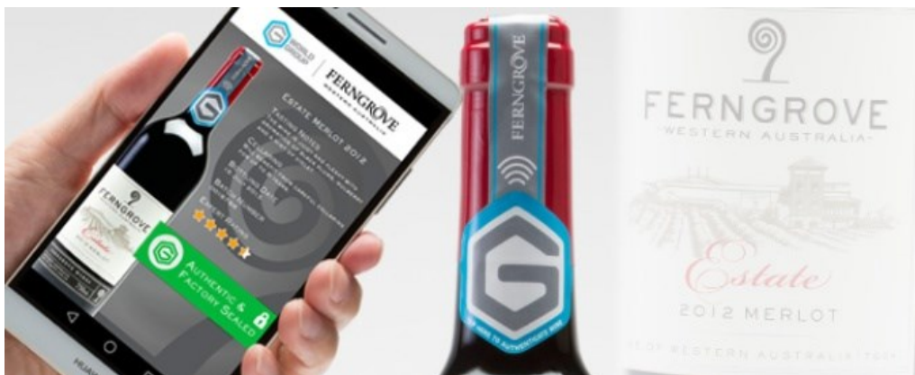
Figure 20: Smart wine bottle by Thinfilm and G World Group. Picture courtesy of Thinfilm.
